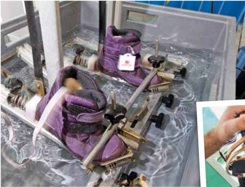
Shoes are also tested in distribution centres. Here, an elephant shoe must prove its resistance to water even under extreme stress.
